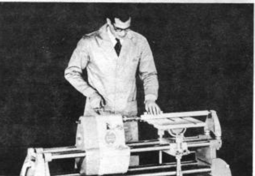
Fig. 57 How to set up for concentric drilling
