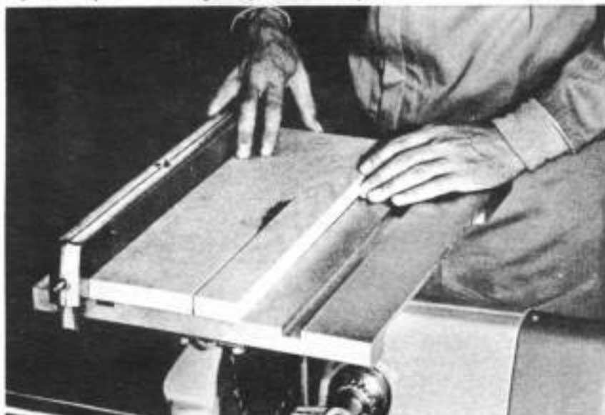
Fig. 20 Hook fingers over fence when ripping
