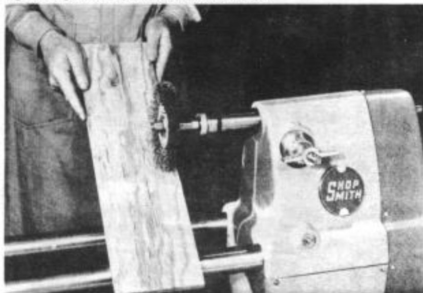
Fig. 61 Wire brushing Fir plywood for sculptured effect
