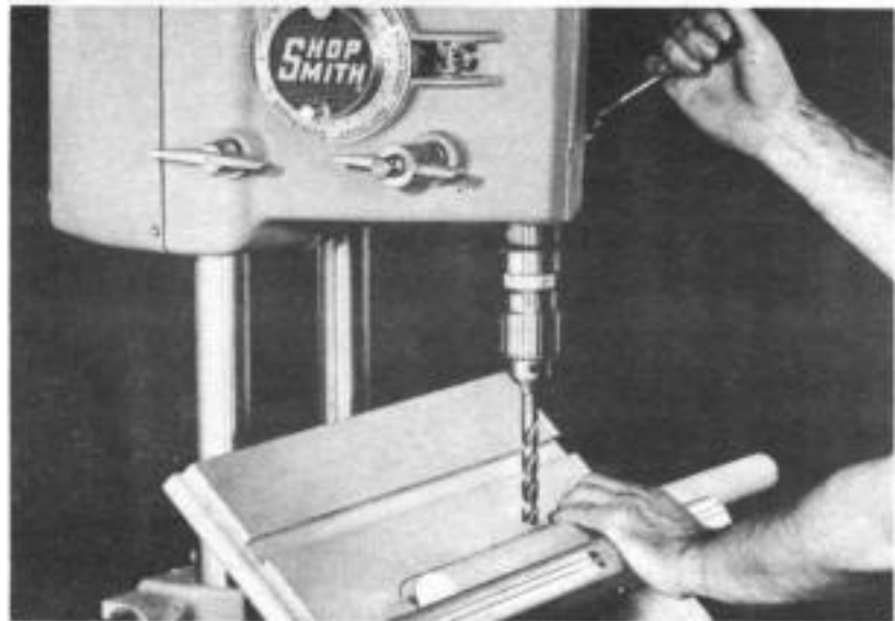
Fig. 44 V-Block jig for drilling round stock
