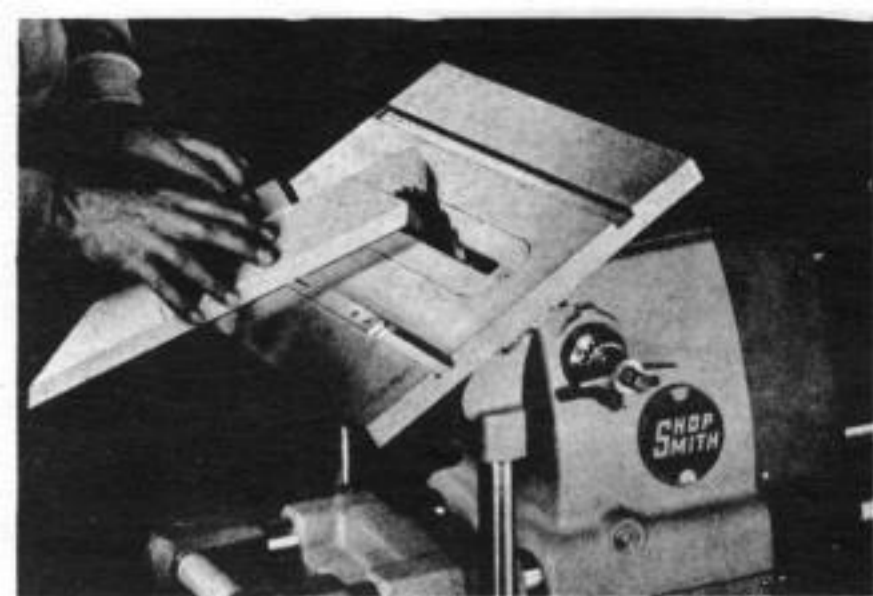
Fig. 25 Compound angle is combination miter and bevel
