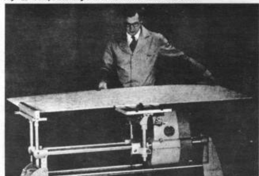
Fig. 26 Plywood panels are easy to cut on SHOPSMITH M5
